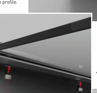
← Align the glass panel and secure it with glass fixings.
